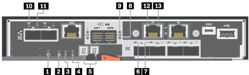
Figure 49. DE6000 controller with quad-port HIC
