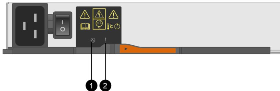
❶ Power LEDs. If it is **Solid green**, the power canister is functioning correctly. If it is **Off**, the power canister failed, the AC switch is turned off, the AC power cord is not properly installed, or the AC power cord input voltage is not within margin (there is a problem at the source end of the AC power cord).
