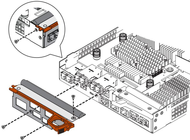
Step 3. Align the three thumbscrews on the HIC with the corresponding holes on the controller, and align the connector on the bottom of the HIC with the HIC interface connector on the controller card. Be careful not to scratch or bump the components on the bottom of the HIC or on the top of the controller card.
