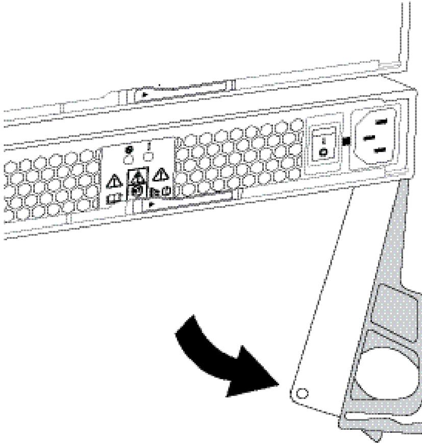
Step 4. Use the cam handle to slide the power supply out of the system.
