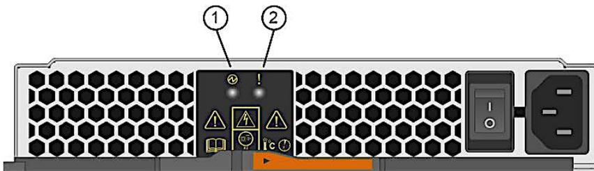
❶ Power LED: If it is **solid green**, the power supply is functioning correctly. If it is **Off**, the power supply failed, the AC switch is turned off, the AC power cord is not properly installed, or the AC power cord input voltage is not within margin (there is a problem at the source end of the AC power cord).
