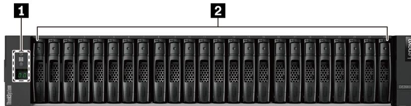
Figure 2. Front view of models with 24 drive bays
