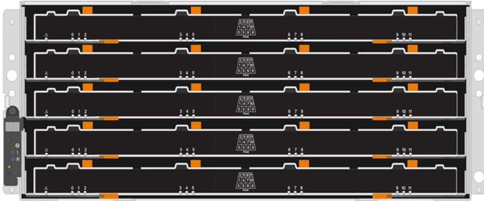
For both a DE4000H/DE6000H controller shelf drawer and a DE600S drive shelf drawer, drives are numbered from 0 to 11 in each drive drawer within the shelf.
