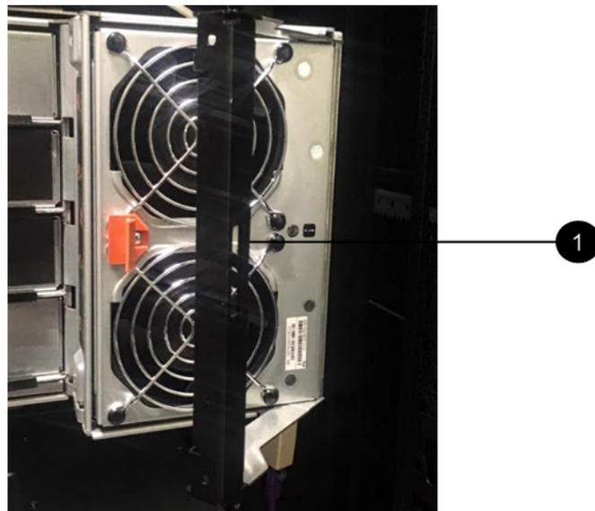
❶ Handle to pull the fan canister out.
