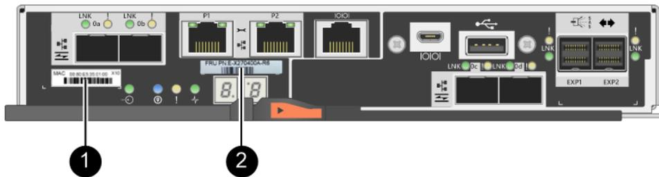
❶ **MAC address:** The MAC address for management port 1 (“P1”). If you used DHCP to obtain the original controller’s IP address, you will need this address to connect to the new controller.
