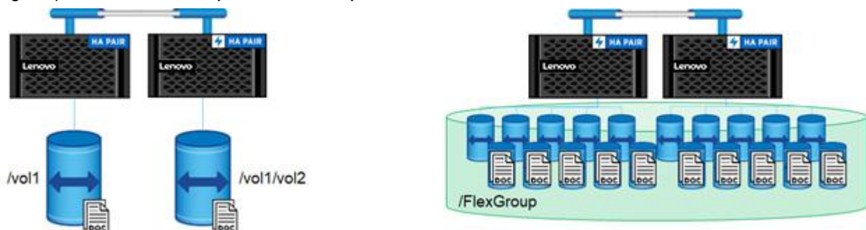
Figure 5) FlexVol and FlexGroup architecture comparison.
