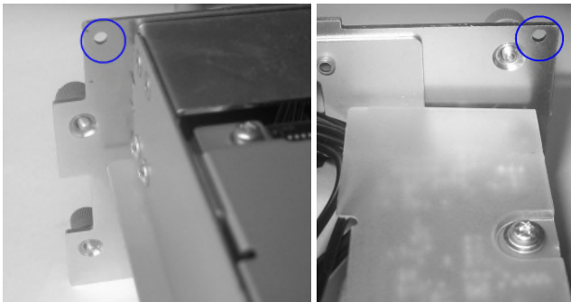
Figure 6 Left - left access hole on the tape drive sled, bottom inside view Right - right access hole on the tape drive sled, bottom inside view
