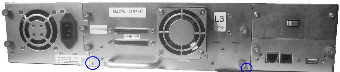
Figure 8 Left and right access holes at the back of the 3362-2LX, highlighted
