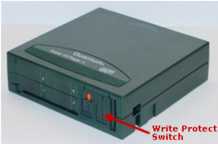
Figure 6: Location of Write Protect Switch
