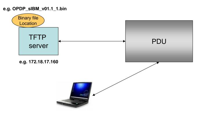
Set up TFTP server IP address and file name for transferring the binary (image) file to PDU (Firmware upgrade) via WEB page.
