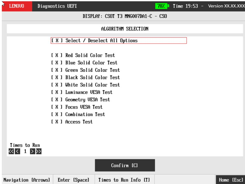
Figure 29: Display algorithm selection
