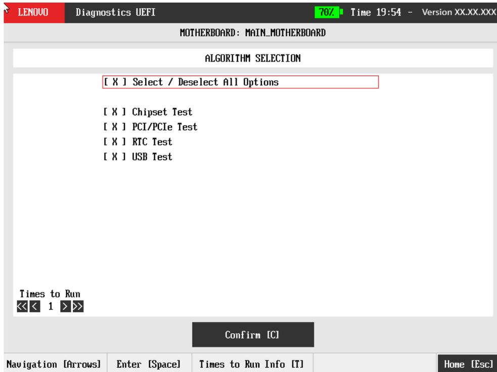
Figure 48: Motherboard algorithm selection
