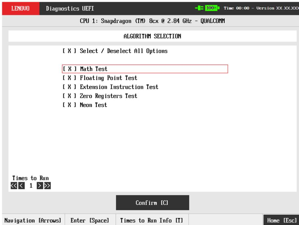
Figure 23: CPU algorithm selection - ARM version
