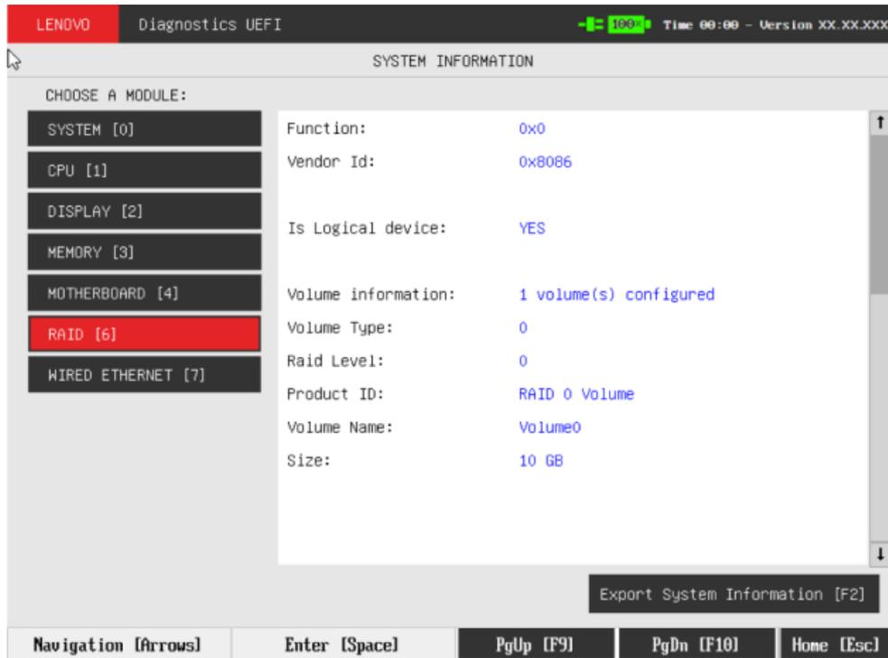
Figure 115: System information - virtual RAID tab
