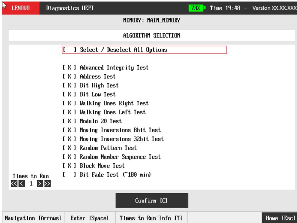
Figure 45: Memory extended algorithm selection
