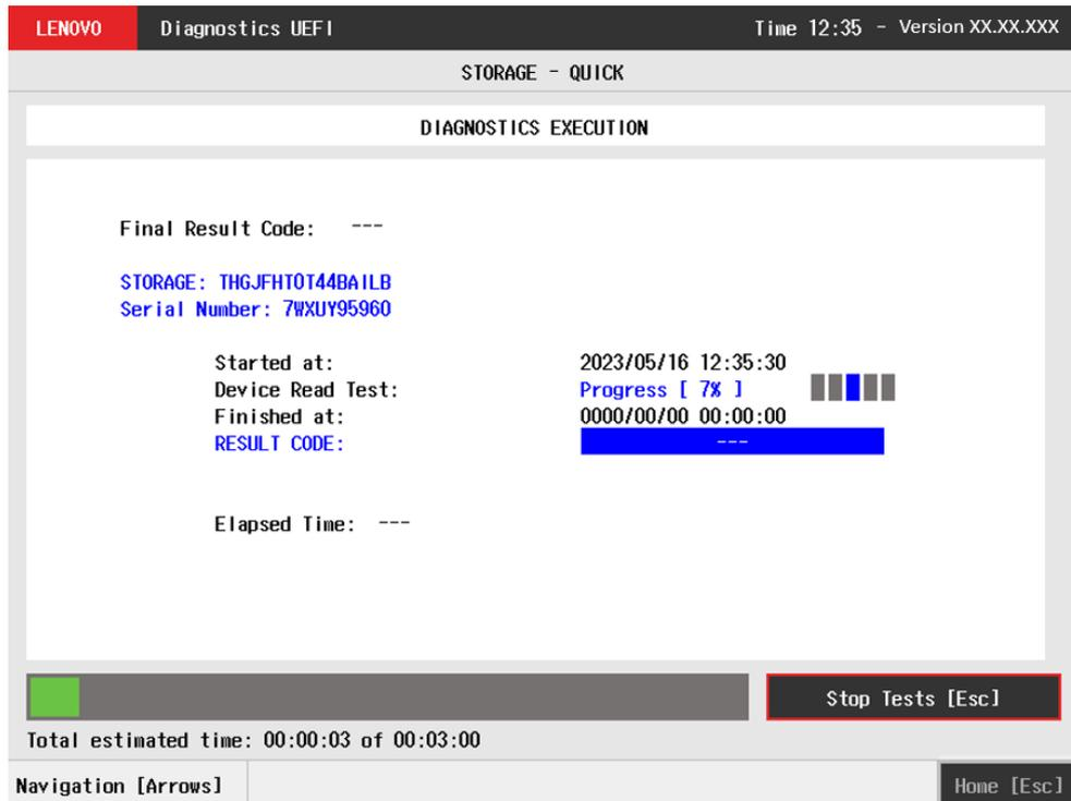
Figure 71: Storage quick diagnostics execution for UFS devices
