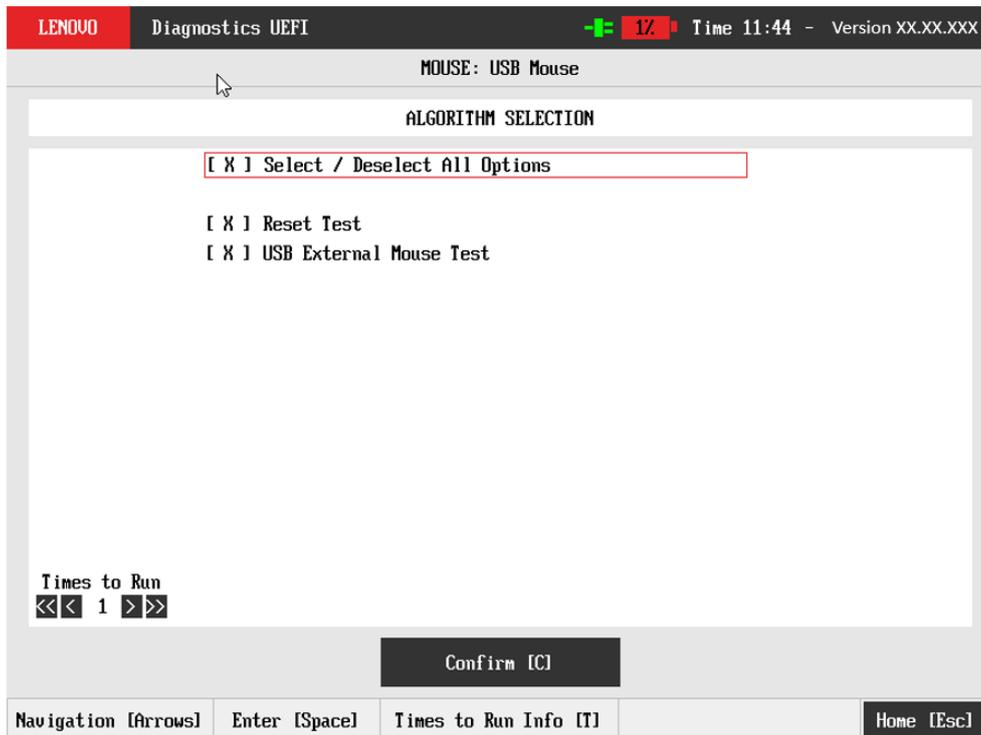
Figure 51: Mouse algorithm selection
