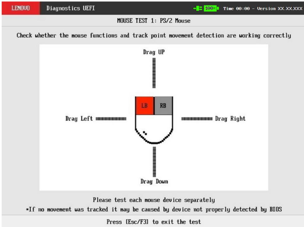
Figure 52: Mouse test execution PS/2
