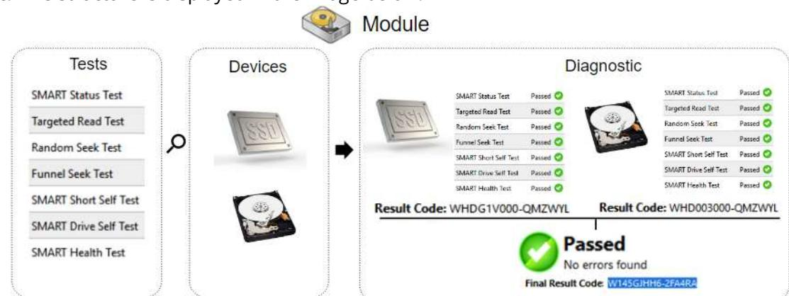
When a diagnostic is finished, Lenovo Diagnostics displays the results for each performed test and creates two results codes resuming the test execution.
