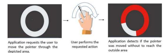
If the user gets to move the pointer through the entire depicted area without reaching the outside area, the test is finished as passed. If the outside area was reached twice, the test will fail. If the pointer is not moved for more than 30 seconds the test will be closed and the following message will be displayed to the user:
