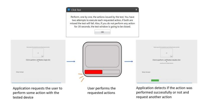
The user must perform one by one, the actions issued by the test. Note that the actions requested depend on the numbers and types of buttons present in your touchpad device.
