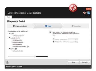
By clicking to Run Tests, the diagnostic script execution screen is displayed, and all supported tests are performed. The unsupported tests that do not have an associated device are filtered on this execution. It is possible to finish the execution anytime by clicking on Stop Test.
