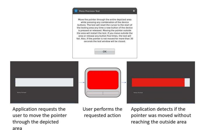
If the user gets to move the pointer through the entire depicted area without reaching the outside area, the test is finished as passed. If the outside area is reached two times the test will fail. If the pointer is not moved for more than 30 seconds the test windows is going to be closed and the following message is displaying to the user:
