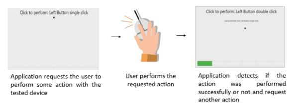
The user must perform one by one, the actions issued by the test. Note that the actions requested depends on the numbers and types of buttons present in your pointing device.
