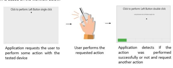
The user must perform one by one, the actions issued by the test. Note that the actions requested depends on the numbers and types of buttons present in your touchpad device.
