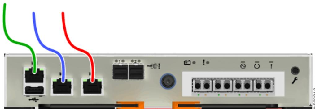
Figure 23. Connecting the Ethernet cables to a Lenovo Storage V5030 system
