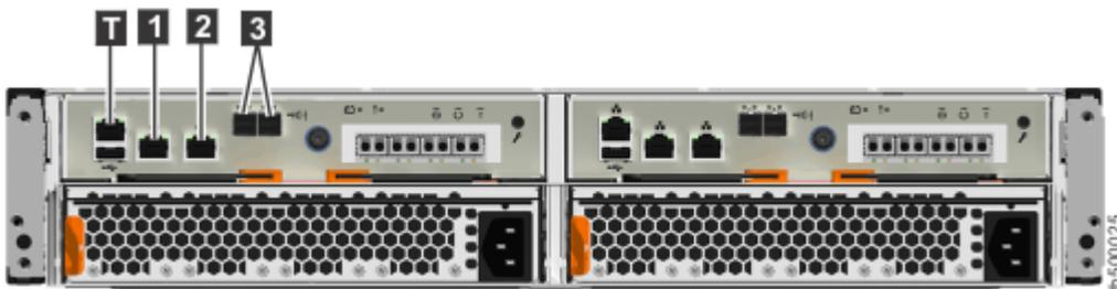
Figure 6. Data ports on the rear of the Lenovo Storage V5030 control enclosure
