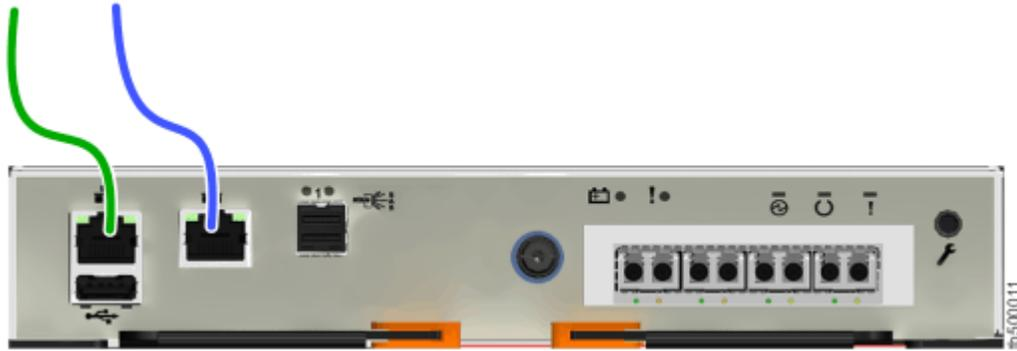
Figure 21. Connecting the Ethernet cables to a Lenovo Storage V3700 V2 system
