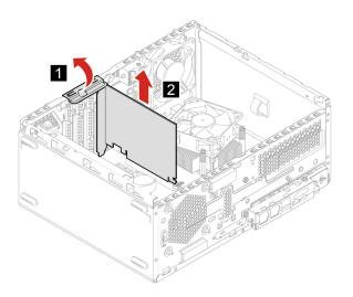
**Note:** If the card is held in place by a retaining latch, press the latch as shown to disengage the latch. Then, gently remove the card from the slot.
