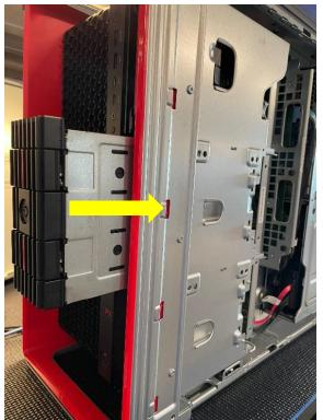
7. Make sure the M.2 SSD Enclosure latched into place as shown below.
