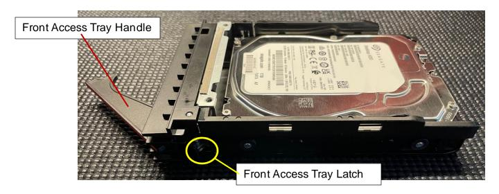
5. Slide the front access HDD tray into the front access bay as shown below.
