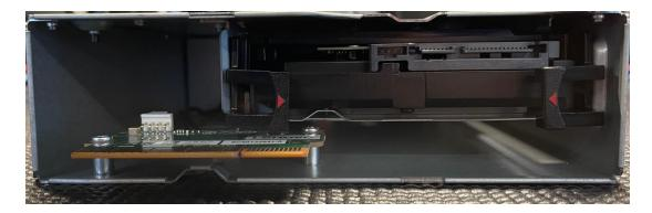
6. Slide the PSU bay storage enclosure into the bottom PSU bay as shown below.
