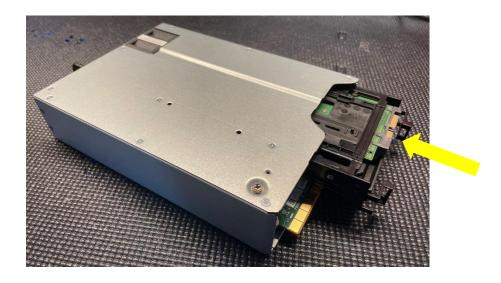
5. Here is what the end of the PSU bay storage enclosure should look like when the drive is fully installed.
