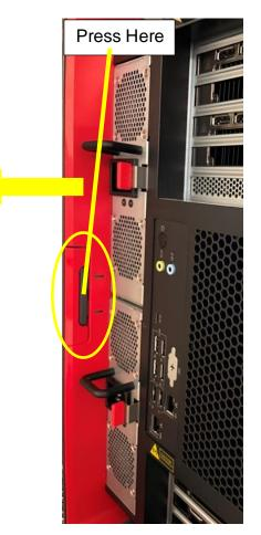
4. While looking at the right side of the system (under the motherboard), press the release tabs to remove the blank bezel for the front access bays 2 and/or 3 depending on how many M.2 storage enclosures to add.
