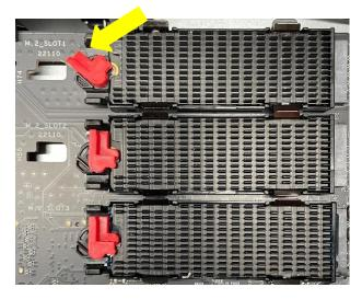
3. Slightly lift straight up to about a 15-degree angle and pull out. Caution: Be careful <u>not</u> to lift too much to risk breaking the M.2 slot.
