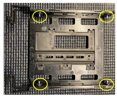
3. Install the 3.5" SATA HDD bottom down in the SATA HDD Tray with the signal and power connections on the same end as the tray handles as shown.
