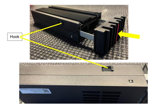
8. Install the M.2 carrier back into the Front Bay Assembly.
