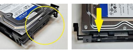
4. Slide the SATA HDD tray back into the PSU bay storage enclosure until it latches into place as shown below.
