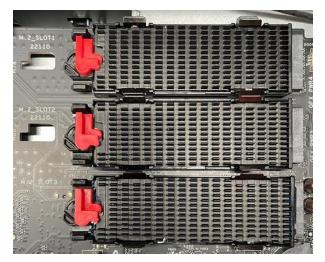
2. Rotate the red locking mechanism counterclockwise.
