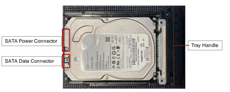
4. Prior to installing the front access tray into the front access bay, make sure the red handle and latch be opened as shown in the picture.
