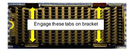
8. Install the M.2 bracket back into the onboard M.2 slot at a slight 15-degree angle.
