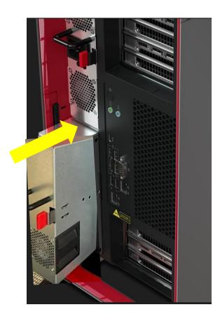
7. Remove the chassis right side door cover to install the SATA signal plus power cable as shown below.
