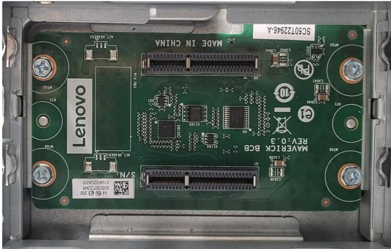
Note: Installing a BCB prevents use of 3.5" SATA drives in the drive storage bays.
