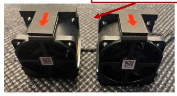
$<sup>^{\</sup>rm 1}$  Memory DIMM fans ( FRU: 5M11H28536) are required when using 3DS RDIMMs or 64GB PC5-5600 MHz RDIMMs.
