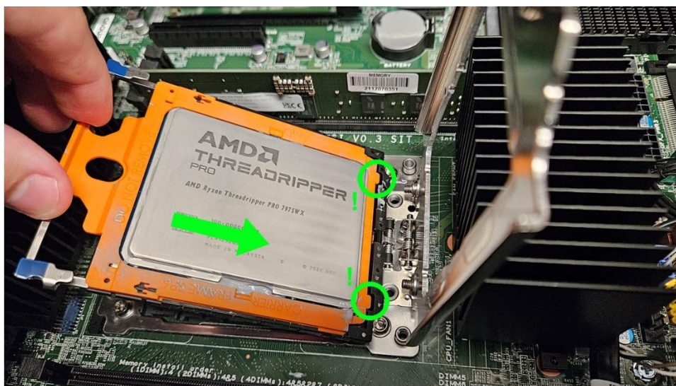
Figure 9 – CPU tray fully inserted into Rail Frame, locks in place.
