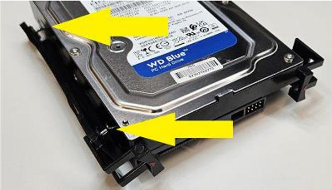
4. Install the drive/tray assembly by fitting the tray into the channels of either of the 3.5" bays. Slide the assembly down until you hear it latch into place.
