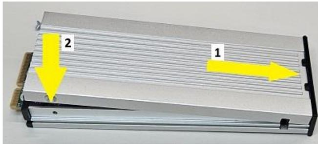
8. Insert the M.2 carrier into the FLEX bay through the front opening. Push firmly until the carrier latches into place in the FLEX bay.
