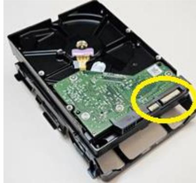
8. Line up the holes on the side of the drive with the posts on the inside of the carrier and insert the posts into the holes.
