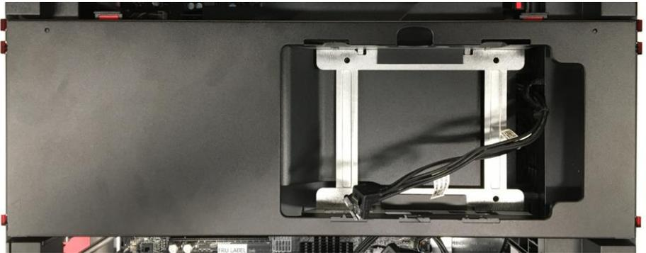
6. The 3<sup>rd</sup> HDD needs to be installed in a special drive carrier before being mounted in the system. Set the drive carrier on a flat surface, upside down, as seen in the below image. Note the position of the red handle.
