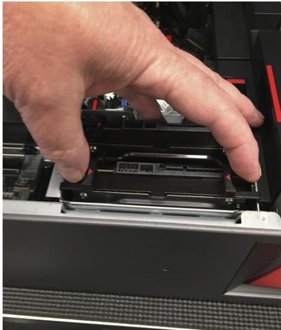
5. Connect the SATA power and data cables as shown in the following photo. One dual drop SATA power cable and one single drop SATA data cable are installed as standard parts in every P7. If you are installing a second 3.5" HDD, you can route the cable to the SATA ports on the motherboard along the same path that the installed power & data cables follow.
