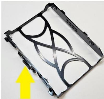
7. Align the drive, upside down, so that the signal and power plugs are on the end of the carrier as seen in the below image.
