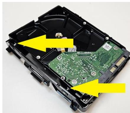
10. Align the tabs on the side of the drive carrier with the notches on the inside of the tray and insert the tabs. Lower the carrier side with the red handle down into the tray and press on the red handle until it clicks into place.
