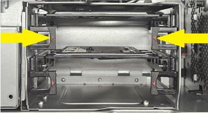
2. Insert the drive, bottom down, into the tray with the signal and power connections on the same end as the arrowed tabs. Angle the side of the drive down into the tray and line up the holes on the side of the drive with the posts on the inside of the tray then insert the posts.
