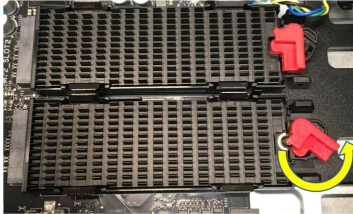
3. Tilt the front side of the M.2 carrier up slightly and pull to the right to remove it from the socket.
