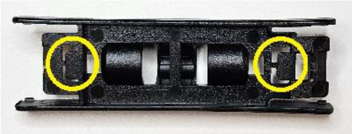
17. Position the carrier to insert the open end of the tabs into the notches on one of the key carrier mount locations. Line up the center guides on the carrier with the openings in the center of the notches
