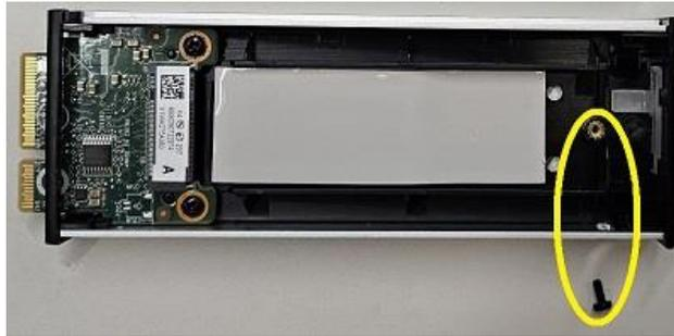
6. Insert the M.2 SSD into the M.2 slot in the carrier base at a slight 15-degree angle (1). Gently lower the M.2 into place with the round notch lining up with the screw hole in the carrier base (2). Reinstall the screw to secure the M.2 drive in the carrier.
