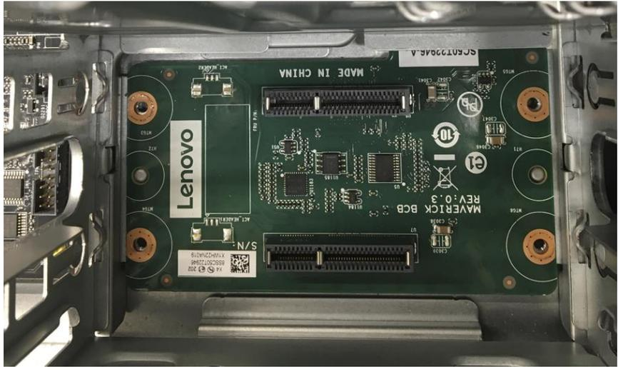
5. Make sure that the card edge connector contacts protrude into the empty cavity just beyond the inside wall of the 3.5" bay:
