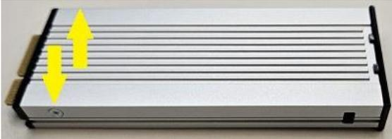
3. Lift up on the lid on the end of the carrier slightly (1) and slide the lid out from under the tabs on the front of the carrier base (2).
