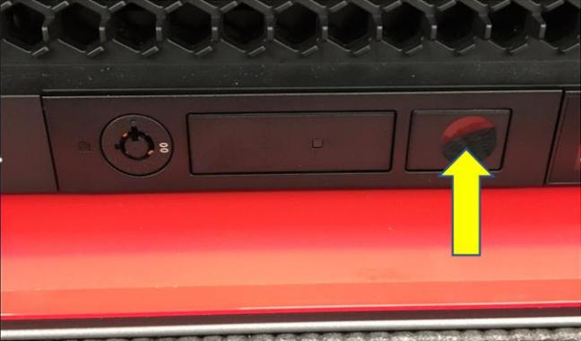
14. The FLEX bay also includes 2 keys in a mountable key carrier. These keys can be used to lock the M.2 carrier into place once it has been inserted.
