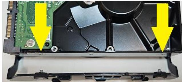
9. Gently bend the open side of the carrier outward, until the posts on the carrier can clear the side of the drive. Then insert the posts into the holes on the side of the drive.
