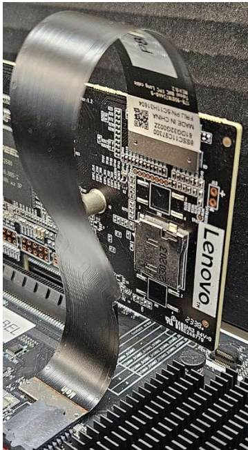
Figure 15, Sideband cable into the BMC card port in the PX
