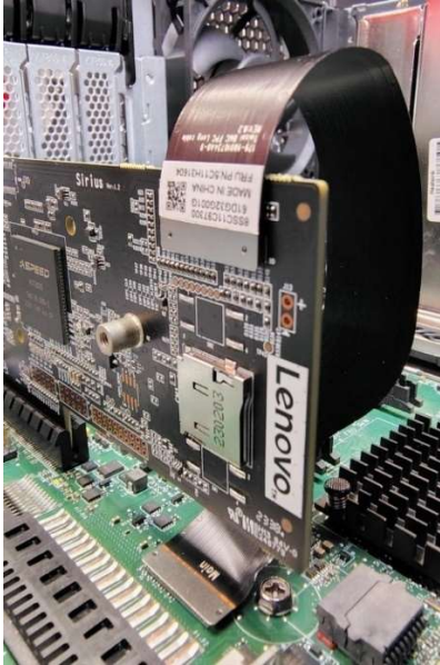
Figure 14, Sideband cable into the BMC card port in the P5, P7, and P8
