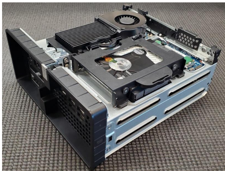
Figure 14 - P3 Ultra Chassis with SATA Bracket Installed
