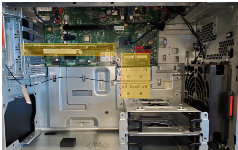
Figure 2 - P3 Tower Chassis with NVMe Callouts
