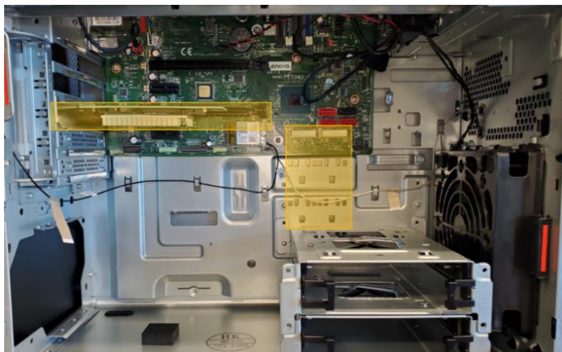
Figure 2 - P3 Tower Chassis with NVMe Callouts
