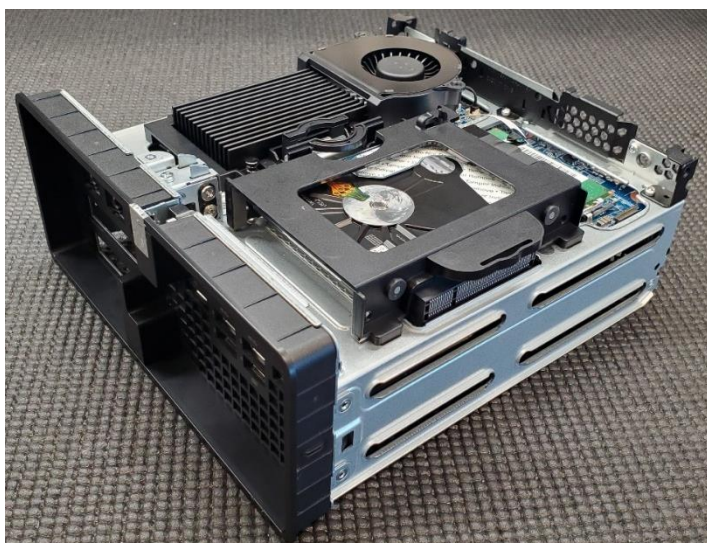
Figure 14 - P3 Ultra Chassis with SATA Bracket Installed
