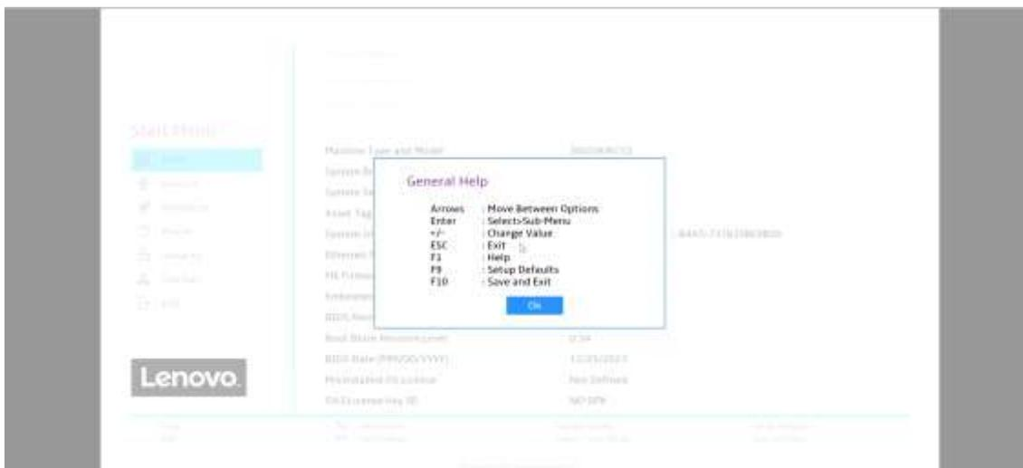
2. Select “System Summary” and scroll down to verify BIOS is recognizing all the drives installed in the system.
