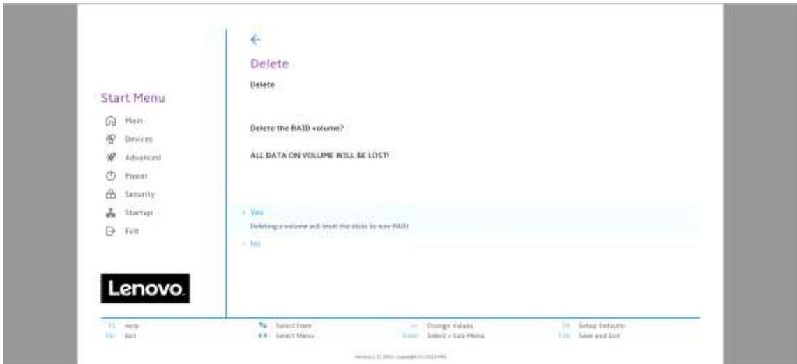
18. To verify the array was deleted, return the opening page of the “Intel(R) Rapid Storage Technology” and verify the drives are once again seen as available for the creation of a new array.
