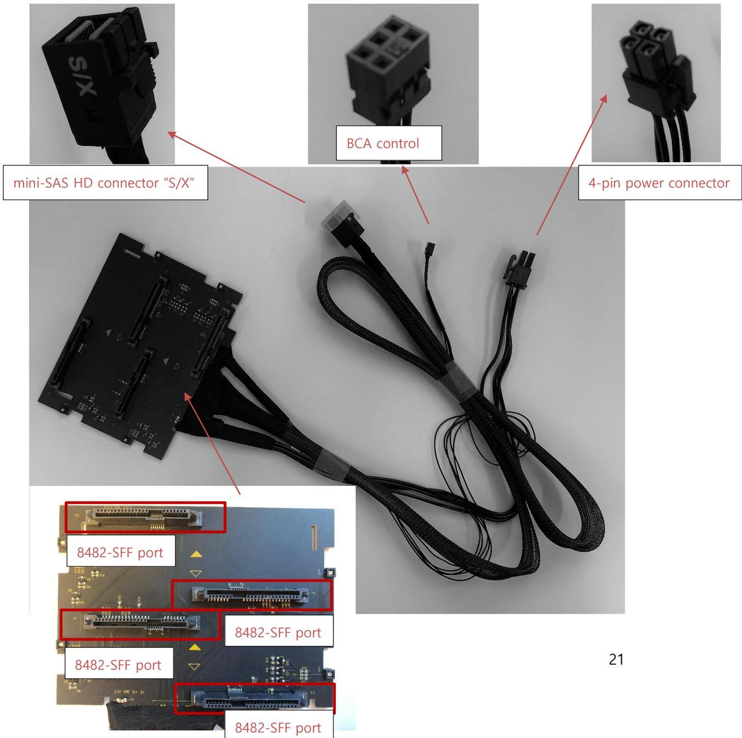
**BCA-P:** Blind Connect Assembly consisting of two 8639-SFF (U.2) ports (supporting PCIe, SAS, or SATA drives) and two 8482-SFF ports (supporting SAS or SATA drives). The assembly also contains the following cable connections:
