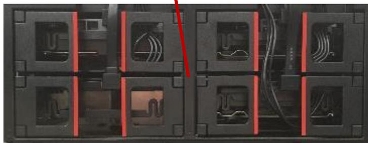
Optionally, in the P720 system, SATA drives can be connected to the onboard Intel SATA controller via BCA's. This consists of the Blind Connect to SATA cable and dual BCA-S. The P720 system can support up to 4 drives using the onboard Intel SATA controller.
