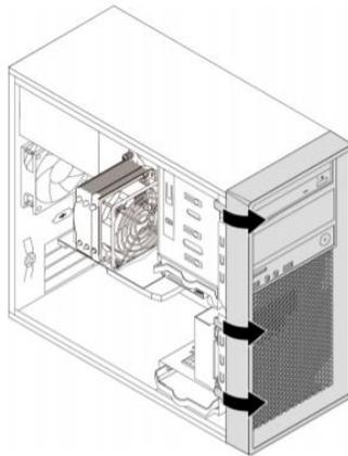
Use the finger cutouts to pull the EMI shield out of the bay.
