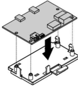
6. Install the retaining bracket/adapter card assembly into the FLEX module by reversing the procedure performed in step 4. Slide the assembly forward until the retention clip snaps into place.
