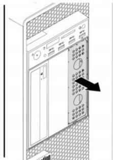
There is an optical drive retainer on the side of the ODD/FLEX bay cage – remove this retainer and install it on the left side of the FLEX module as shown here:
