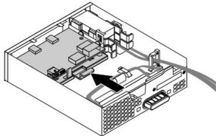
7. Plug four cables into the rear of the adapter card. The power cable is already part of the FLEX module and the remaining 3 cables were supplied with the Thunderbolt 3 kit. Use the following connector layout diagram as a guide for cable connections:
