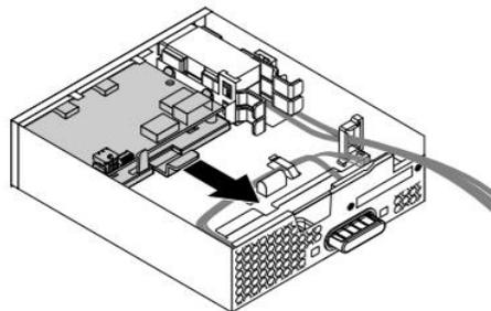
5. Install the Thunderbolt I/O adapter card onto the retaining bracket by aligning the four locator holes with the corresponding mounting posts on the bracket. Press down on the card until the four retaining clips snap into place, securely mating the two parts into a single assembly.
