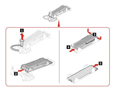
Note: When installing the M.2 solid-state drive and the heat sink, remove the film that covers the thermal pad (if any).
