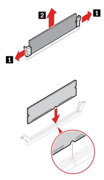
Note: During the installation, ensure that you align the memory module to the slot and press down on both ends until the latches are fully engaged with a click.
