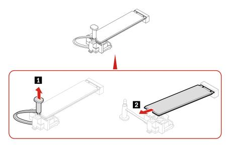
• For computers with the heat sink for the M.2 solid-state drive:
