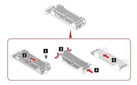
**Note:** When installing the M.2 solid-state drive and the heat sink, remove the film that covers the thermal pad (if any).
