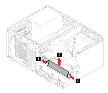
Note: During the installation, ensure that you align the memory module to the slot and press down on both ends until the latches are fully engaged with a click.
