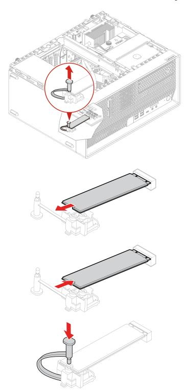
• For computers with the heat sink for the M.2 solid-state drive:
