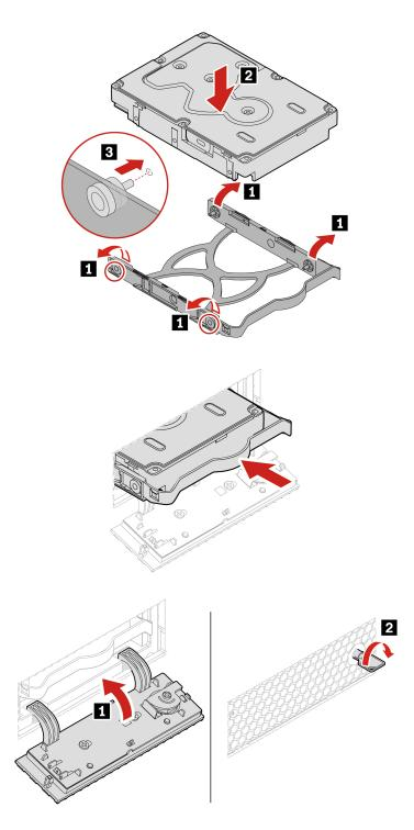
Replacement procedure for 2.5-inch storage drive installed in the 3.5-inch front-access storage enclosure through Type-2 storage drive converter
