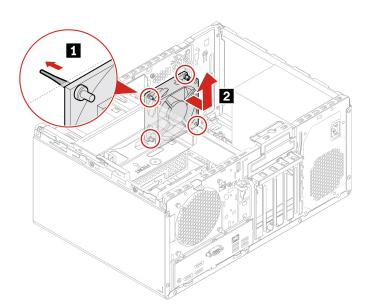
**Note:** The front fan is attached to the chassis by four rubber mounts. Stretch the tips of the rubber mounts and gently pull the front fan assembly out of the chassis.
