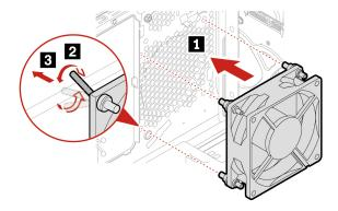
**Note:** Align the rubber mounts with the corresponding holes in the chassis and push the rubber mounts through the holes. Rotate and pull the tips of the rubber mounts until the front fan assembly is secured.
