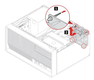
**Note:** The rear fan is attached to the chassis by four rubber mounts. Stretch the tips of the rubber mounts and gently pull the rear fan assembly out of the chassis.
