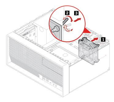
**Note:** Align the rubber mounts with the corresponding holes in the chassis and push the rubber mounts through the holes. Rotate and pull the tips of the rubber mounts until the rear fan assembly is secured.
