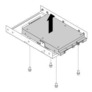
Figure 104. Removing the 2.5-inch storage drive from the storage-drive converter
