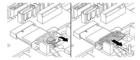
Figure 144. Pulling handle of the retention latch outward and removing the shield
