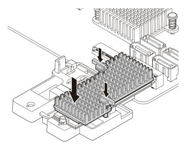
Figure 40. Installing the heat sink onto the plastic holder
