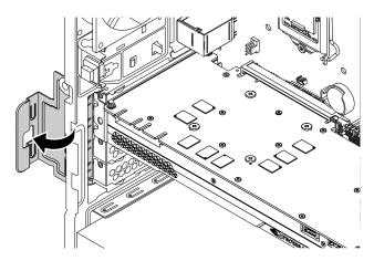
Figure 29. Rotating the PCIe card retainer
