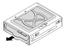
Figure 97. Removing the 3.5-inch storage drive
