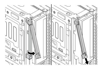
Figure 20. Removing the metal shield
