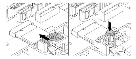
Figure 138. Reinstalling the shield and insert the plug of the retention latch into the hole to secure the Wi-Fi card module
