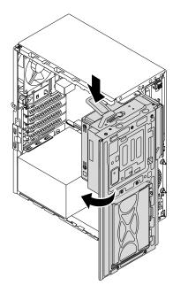
Figure 176. Pivoting the drive bay assembly downward
