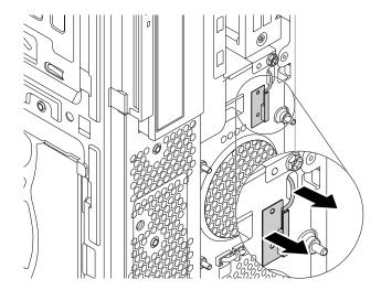
Figure 140. Removing the front Wi-Fi antenna cable
