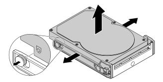
Figure 57. Removing the 3.5-inch storage drive from the bracket
