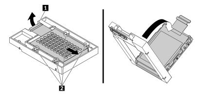
Figure 63. Removing the adapter from the converter
