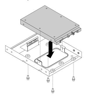
Figure 93. Installing the new 2.5-inch storage drive into the storage-drive converter
