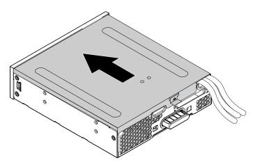
Figure 163. Reinstalling the flex module cover
