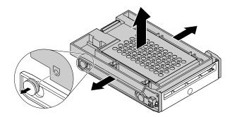
Figure 62. Removing the 2.5-inch storage drive from the bracket
