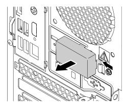
Figure 145. Removing the shield
