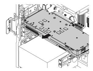
Figure 30. Removing a full-length PCIe card
