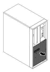
Figure 13. Removing the dust shield
