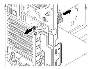
Figure 84. Removing the cover presence switch
