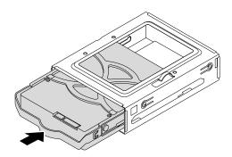
Figure 99. Installing the storage drive
