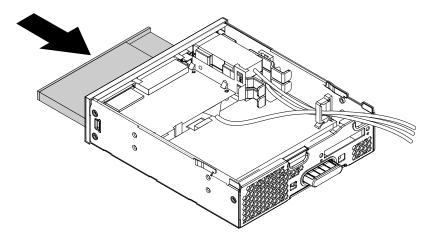
Figure 162. Installing the slim optical drive into the flex module
