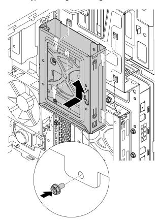
Figure 108. Installing the type-1 storage-drive cage
