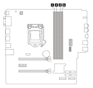
Figure 47. Memory module installation sequence
