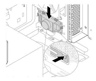
Figure 129. Removing the internal speaker
