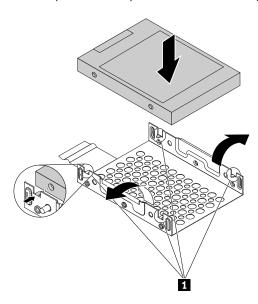
Figure 65. Installing the storage drive into the adapter
