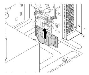
Figure 130. Installing the internal speaker
