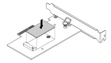
Figure 44. Installing the thermal pad
