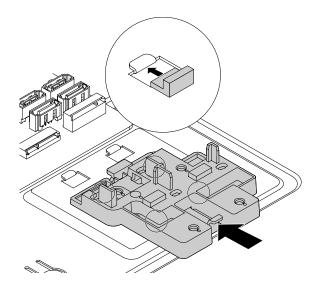
Figure 37. Installing the plastic holder
