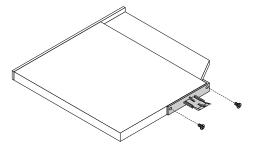
Figure 161. Installing the plastic clip to the slim optical drive
