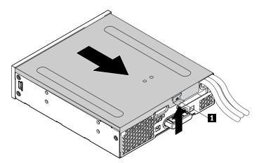
Figure 164. Removing the flex module cover
