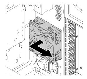
Figure 122. Removing the front fan
