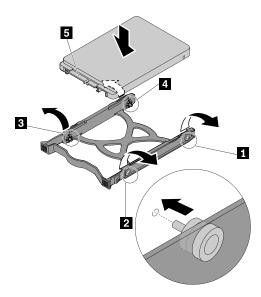
Figure 111. Installing the 2.5-inch storage drive into the bracket
