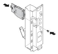
Figure 120. Installing the card reader
