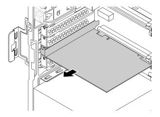
Figure 25. Removing a PCIe card
