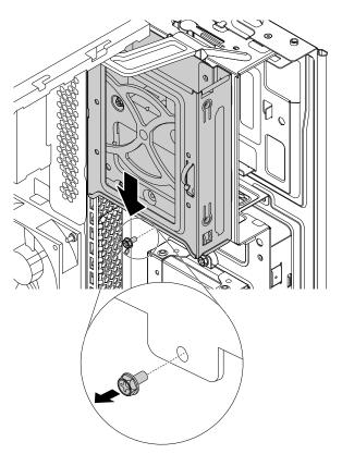
Figure 101. Removing the type-1 storage-drive cage
