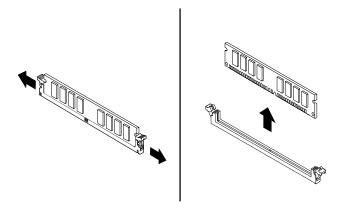
Figure 48. Removing a memory module
