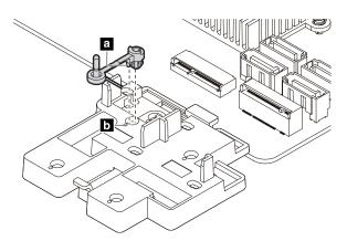
Figure 135. Installing the retention latch
