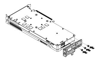
Figure 32. Installing a full-length PCle card bracket
