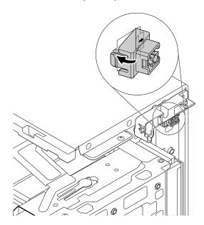
Figure 115. Installing the power button
