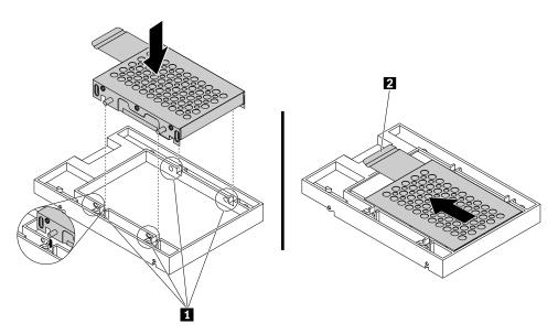
Figure 66. Installing the adapter into the converter
