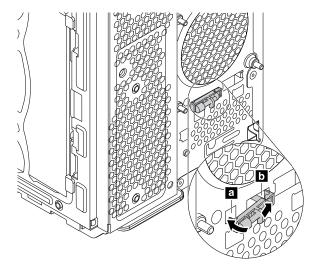
Figure 128. Installing the thermal sensor
