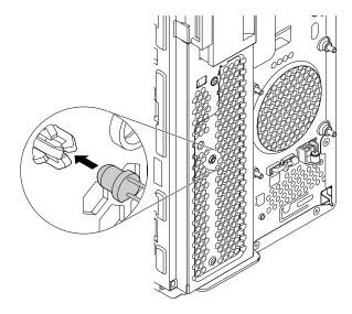
Figure 117. Installing the ThinkStation LED
