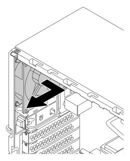
Figure 124. Removing the rear fan
