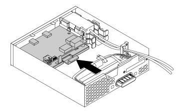
Figure 173. Installing the front Thunderbolt adapter and the retaining bracket into the flex module
