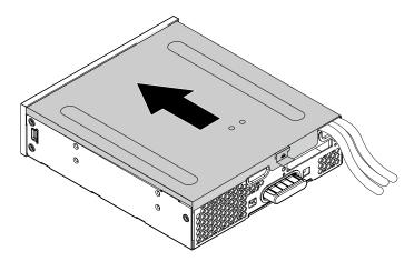
Figure 167. Reinstalling the flex module cover
