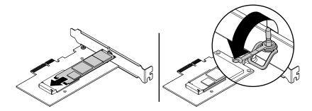
Figure 45. Installing the M.2 solid-state drive
