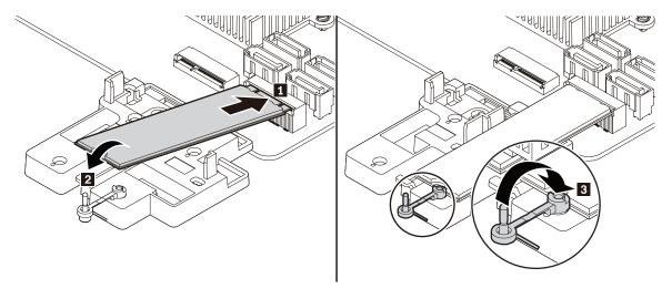
Figure 39. Installing the M.2 solid-state drive
