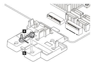
Figure 38. Installing the retention latch
