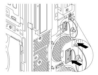
Figure 142. Installing the front Wi-Fi antenna
