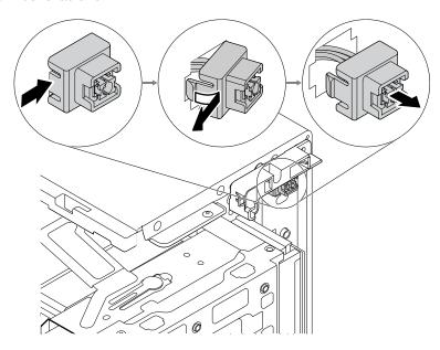
Figure 114. Removing the power button
