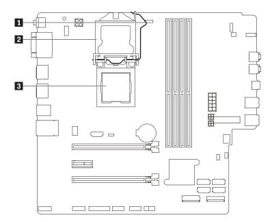
Figure 151. Accessing the microprocessor
