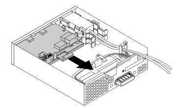
Figure 169. Removing the front Thunderbolt adapter and the retaining bracket out of the flex module
