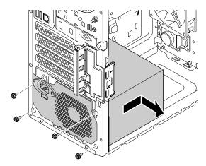
Figure 86. Removing the power supply assembly
