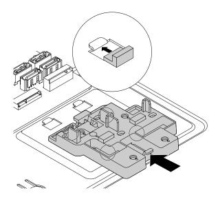
Figure 134. Installing the plastic holder
