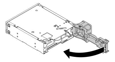
Figure 81. Pivoting the rear cover inward
