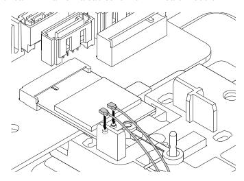
Figure 137. Connecting the front and rear Wi-Fi antenna cables to the Wi-Fi card module
