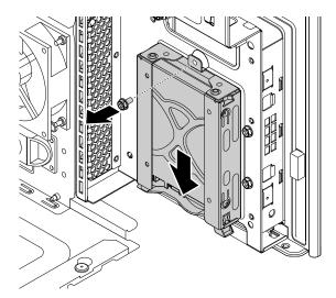
Figure 109. Removing the type-2 storage-drive cage
