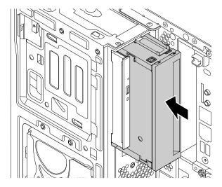
Figure 54. Installing the new flex storage enclosure
