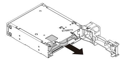
Figure 75. Removing the 2.5-inch storage drive from the rear
