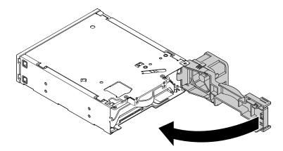
Figure 73. Pivoting the rear cover inward
