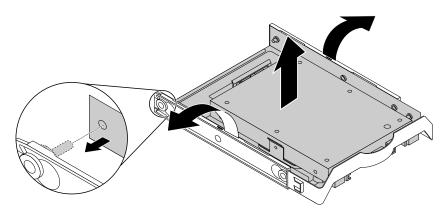
Figure 91. Removing the storage-drive converter from the 3.5-inch storage-drive bracket
