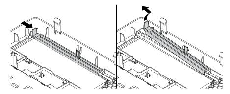
Figure 19. Removing the plastic shield
