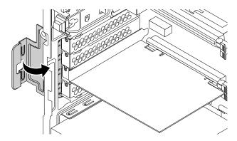
Figure 27. Rotating the PCIe card retainer
