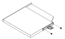
Figure 159. Removing the plastic clip from the slim optical drive
