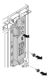
Figure 118. Removing the front audio and USB assembly
