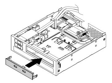
Figure 171. Installing the bezel to the flex module
