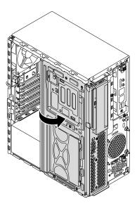
Figure 16. Pivoting the drive bay assembly outward
