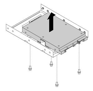
Figure 77. Removing the 2.5-inch storage drive from the storage-drive converter
