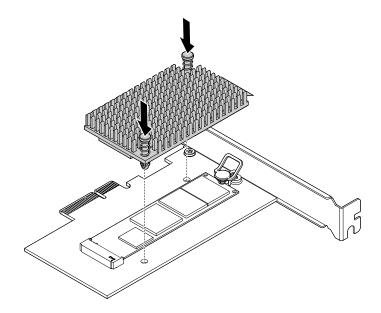
Figure 46. Installing the heat sink
