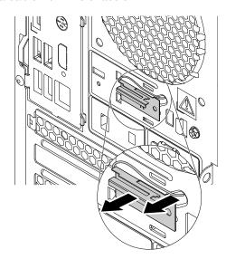
Figure 146. Removing the rear Wi-Fi antenna cable
