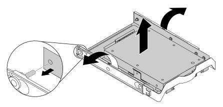
Figure 76. Removing the storage-drive converter from the 3.5-inch storage-drive bracket
