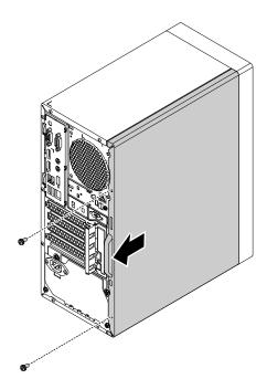
Figure 14. Removing the computer cover
