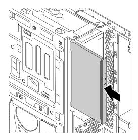
Figure 22. Installing the slim optical drive
