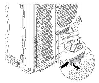
Figure 127. Removing the thermal sensor
