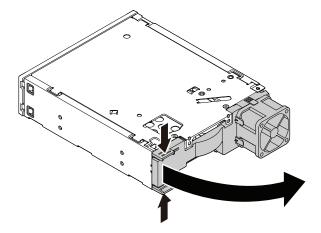
Figure 74. Opening the enclosure from the rear
