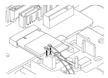
Figure 132. Disconnecting the front and rear Wi-Fi antenna cables from the Wi-Fi card module
