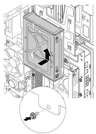
Figure 100. Installing the type-1 storage-drive cage
