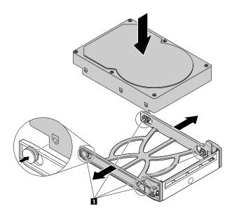
Figure 58. Installing the 3.5-inch storage drive into the bracket
