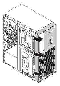
Figure 15. Removing the front bezel
