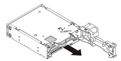
Figure 70. Removing the 3.5-inch storage drive from the rear
