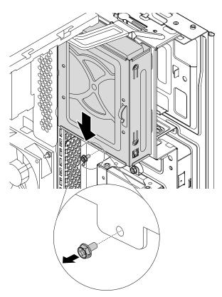
Figure 96. Removing the type-1 storage-drive cage
