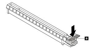
Figure 23. Disengaging the card retaining latch
