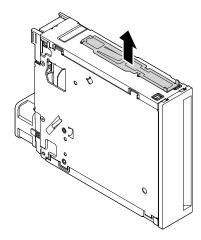
Figure 52. Removing the retainer
