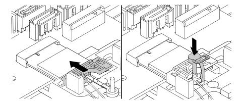
Figure 150. Reinstalling the shield and insert the plug of the retention latch into the hole to secure the Wi-Fi card module
