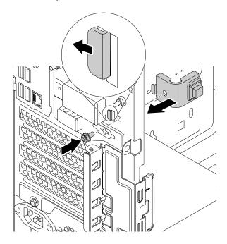
Figure 85. Installing the cover presence switch
