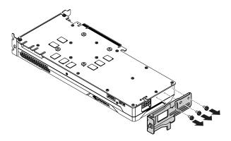
Figure 31. Removing a full-length PCIe card bracket
