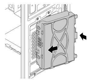
Figure 89. Installing the storage-drive
