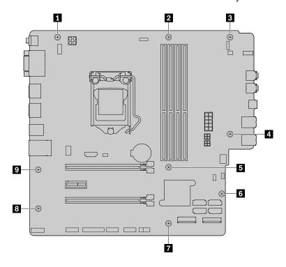
Figure 154. Removing the nine screws that secure the system board
