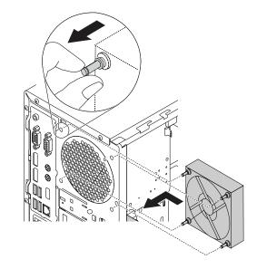
Figure 125. Installing the rear fan
