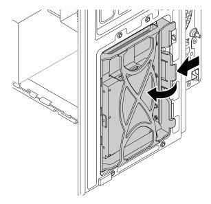
Figure 90. Removing the 2.5-inch storage drive with 3.5-inch storage-drive bracket
