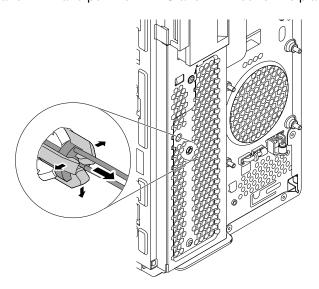
Figure 116. Removing the ThinkStation LED
