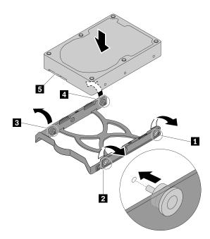
Figure 98. Installing the storage drive into the bracket
