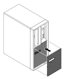
Figure 179. Reinstalling the dust shield
