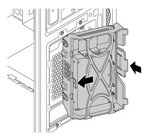
Figure 95. Installing the 2.5-inch storage drive
