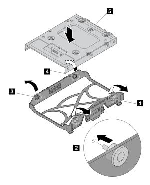
Figure 94. Installing the 2.5-inch storage drive with the storage-drive converter into the bracket
