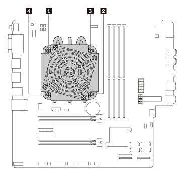
Figure 126. Removing the heat-sink-and-fan assembly
