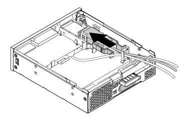
Figure 166. Installing the eSATA connector or IEEE 1394 connector in the flex module
