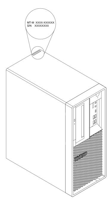
Figure 8. Machine type and model label
