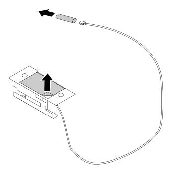
Figure 147. Peeling off the paper that protects the sticker and removing the plastic cover
