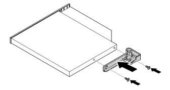
Figure 21. Installing the bracket
