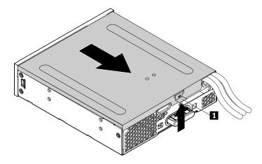
Figure 157. Removing the flex module cover
