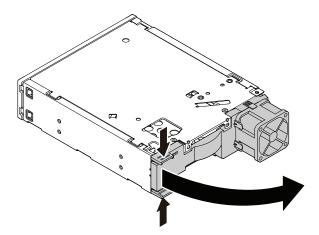
Figure 69. Opening the enclosure from the rear
