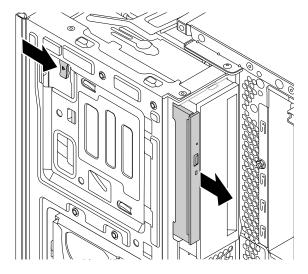
Figure 17. Removing the slim optical drive
