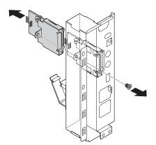
Figure 119. Removing the card reader
