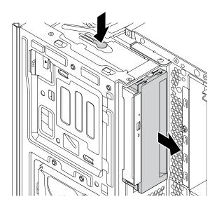
Figure 51. Removing the flex storage enclosure
