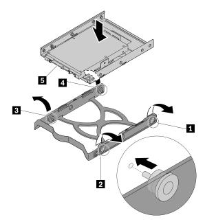
Figure 106. Installing the 2.5-inch storage drive into the bracket
