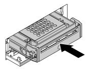
Figure 68. Installing the plastic bracket with the 2.5-inch storage drive into the front-access storage enclosure
