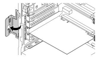
Figure 24. Rotating the PCIe card retainer
