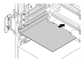
Figure 26. Installing a new PCIe card
