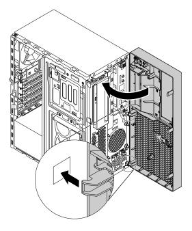
Figure 177. Reinstalling the front bezel
