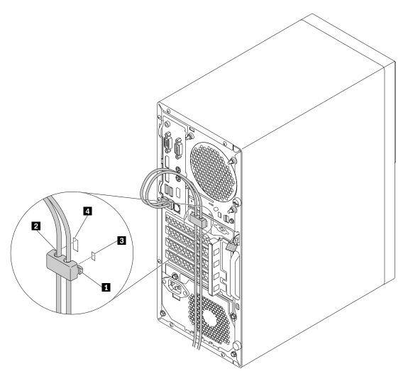
Figure 12. Installing a cable lock
