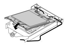
Figure 156. Installing the microprocessor socket cover
