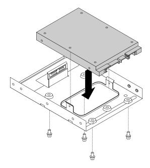
Figure 78. Installing the new solid-state drive into the storage converter
