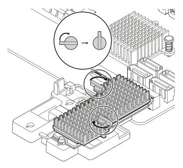
Figure 41. Securing the heat sink to the plastic holder
