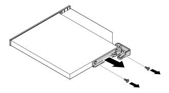
Figure 18. Removing the bracket
