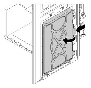
Figure 87. Removing the storage drive
