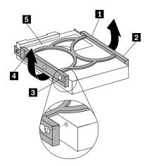
Figure 71. Installing the 3.5-inch storage drive into the bracket
