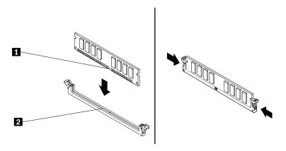
Figure 50. Installing a memory module
