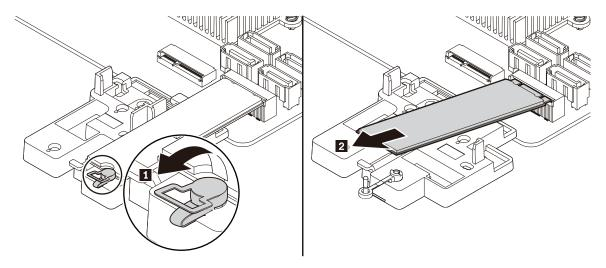
Figure 36. Opening the retention latch and removing the M.2 solid-state drive
