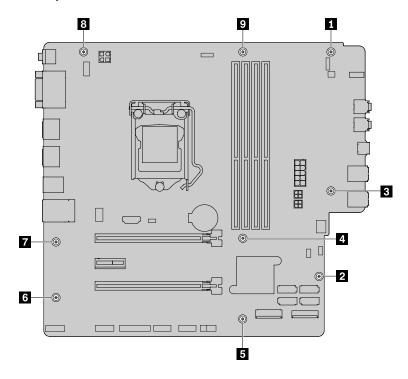
Figure 155. Installing the nine screws to secure the system board
