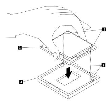
Figure 153. Installing the microprocessor
