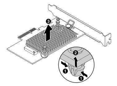
Figure 42. Removing the heat sink from the M.2 solid-state drive adapter
