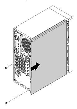
Figure 178. Reinstalling the computer cover
