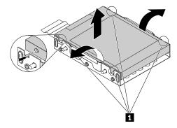
Figure 64. Removing the storage drive from the adapter
