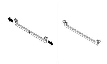
Figure 49. Opening the retaining clips
