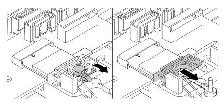
Figure 139. Pulling handle of the retention latch outward and removing the shield
