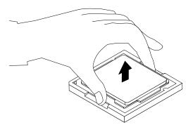
Figure 152. Removing the microprocessor
