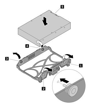
Figure 88. Installing the storage drive into the bracket
