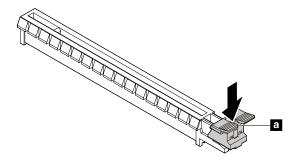
Figure 28. Disengaging the card retaining latch
