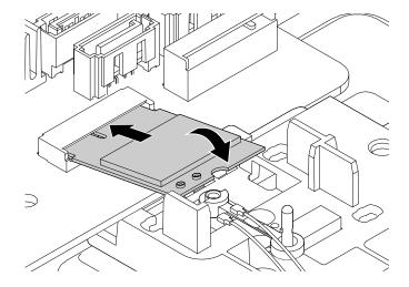
Figure 136. Installing the Wi-Fi card module
