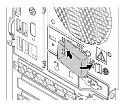
Figure 149. Installing the shield
