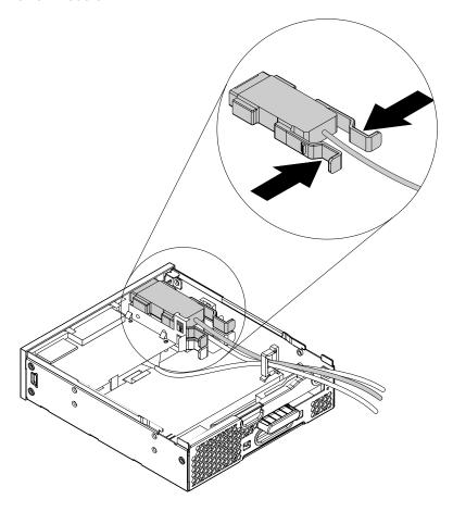
Figure 165. Removing the eSATA connector or IEEE 1394 connector from the flex module
