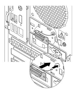
Figure 148. Installing the rear Wi-Fi antenna
