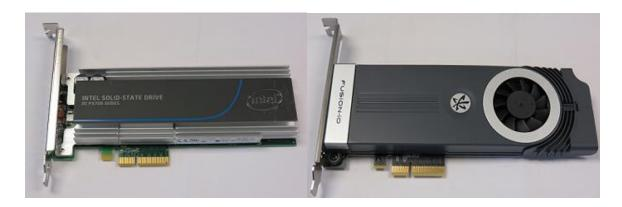
These form factors are all quite different from one another in physical appearance; however their main function is still the same. They are all devices consisting of an onboard controller with onboard solid state memory that use the system's PCIe bus to communicate back to the system processor or chipset.
