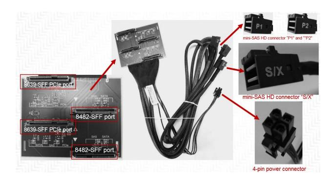
BCA-S: Blind Connect Assembly consisting of four 8482-SFF ports (supporting SAS or SATA drives). The assembly also contains the following cable connections:
