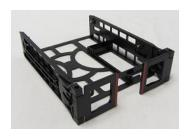
Manual Connect FLEX Tray: Tool-less tray that can hold up to two drives. These trays utilize hinged pulls that open and allow for cable access and manual cable connections.
