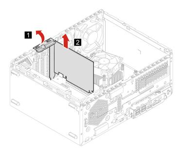
**Note:** If the card is held in place by retaining latch, press the latch as shown to disengage the latch, Then, gently remove the card from the slot.
