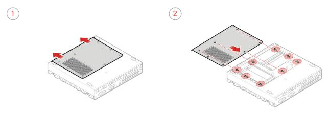
Reinstall the computer cover and reconnect the cables. For details, see *Completing the parts* replacement.
