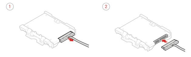
Reinstall the removed parts and computer cover. For details, see *Completing the parts replacement.*
