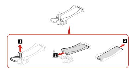
**Note:** Remove the film that covers the thermal pad (if any) when installing the M.2 solid-state drive and the heat sink.
