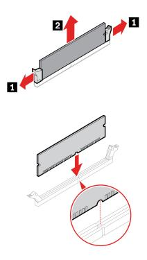
**Note:** During the installation, ensure that you align the memory module with the slot and press down on both ends until the latches are fully engaged with a click.
