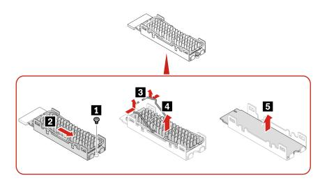
Note: Remove the film that covers the thermal pad (if any) when installing the M.2 solid-state drive and the heat sink.
