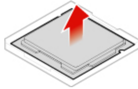
Figure 113. Pivoting the microprocessor socket upward
