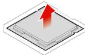
Figure 116. Pivoting the microprocessor socket upward
