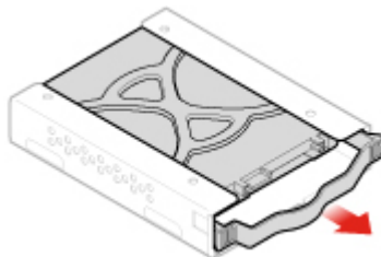
Figure 42. Removing the 2.5-inch secondary storage drive bracket
