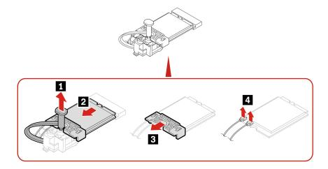
Note: During installation, ensure that you connect the gray cable to the connector labeled AUX on the card, and the black cable to the connector labeled MAIN.
