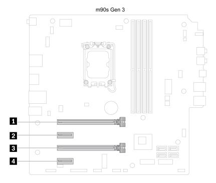
• Before installing a new PCI-Express card, remove any PCI-Express connector cables that impede the installation. See "PCI-Express connector cable" on page 68.
