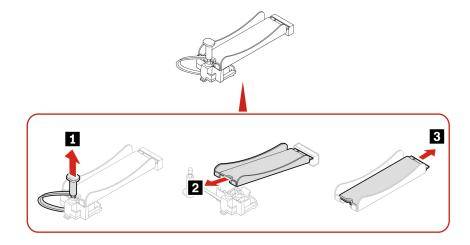
Note: Remove the film that covers the thermal pad (if any) when installing the M.2 solid-state drive.
