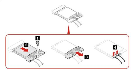
**Note:** While installing, ensure that you connect the gray cable to the connector labeled 1 (auxiliary) and the black cable to connector labeled 2 (main) on the card.
