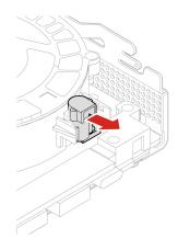
4. Disconnect the system fan cable from the system fan connector on the system board.
