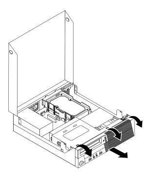
Figure 26. Removing the front bezel
