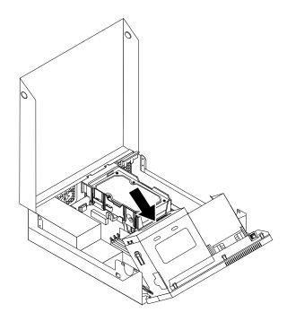
Figure 20. Installing a new optical drive
