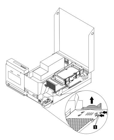
Figure 29. Removing the internal speaker
