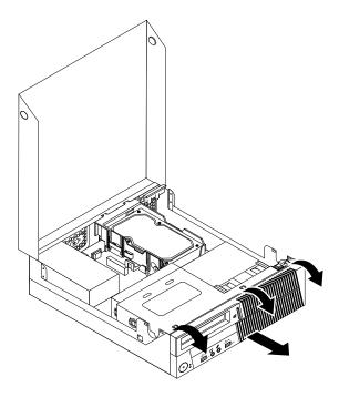
Figure 28. Removing the front bezel
