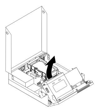
Figure 7. Pivoting the optical drive bay assembly
