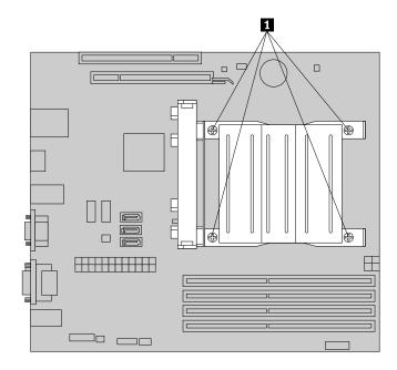
Figure 24. Removing the heat sink
