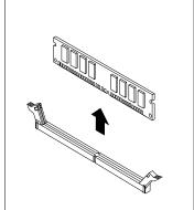
Figure 9. Removing a memory module
