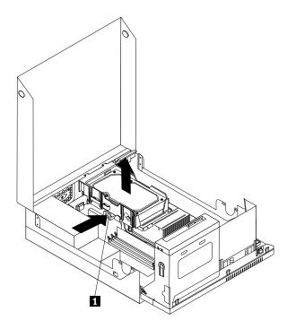
Figure 15. Removing the hard disk drive
