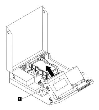
Figure 18. Removing the old optical drive
