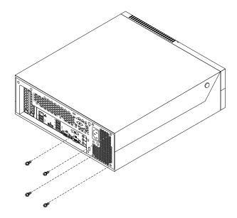
Figure 21. Removing the retaining screws for the power supply assembly
