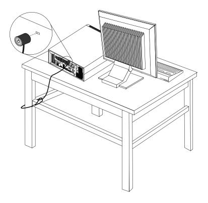
Figure 33. Integrated cable lock
