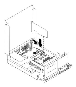
Figure 12. Installing the PCI card
