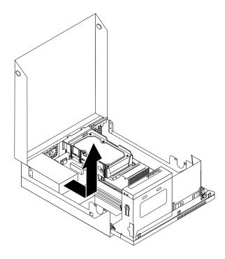
Figure 23. Removing the power supply assembly
