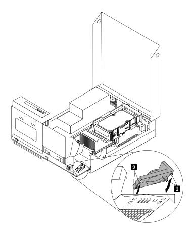
Figure 30. Installing the new internal speaker
