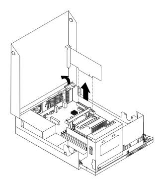
Figure 11. Removing a PCI card
