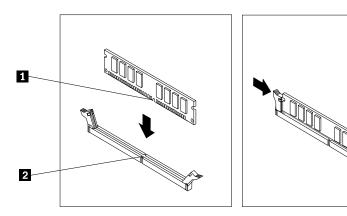
Figure 10. Installing a memory module
