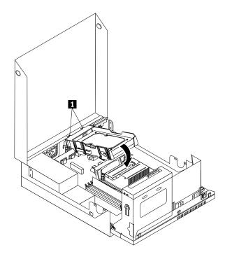
Figure 17. Installing the hard disk drive
