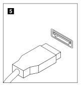
1 USB connector Used to attach a device that requires a USB connector, such as a USB keyboard,
