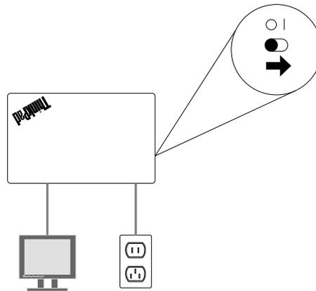
Figure 6. Sliding the power switch on the wireless display adapter to the on position
