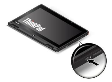
In the tablet mode, the keyboard, the trackpad, and the TrackPoint pointing stick are automatically disabled. However, you can control some functions of your computer through the special buttons and the multi-touch screen, without the use of the keyboard and the touch pad. For more information, refer to "Using the special buttons" on page 17 and "Using the multi-touch screen" on page 18.
