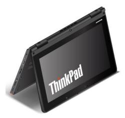
In the tent mode, the keyboard, the trackpad, and the TrackPoint pointing stick are automatically disabled. However, you can control some functions of your computer through the special buttons and the multi-touch screen, without the use of the keyboard and the touch pad. For more information, refer to "Using the special buttons" on page 17 and "Using the multi-touch screen" on page 18.
