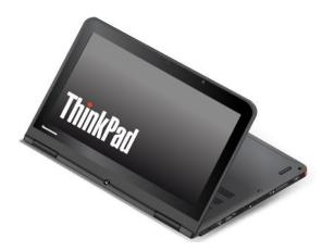
In the stand mode, the keyboard, the trackpad, and the TrackPoint pointing stick are automatically disabled.
