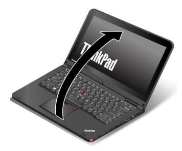
In the notebook mode, the keyboard, the trackpad, and the TrackPoint pointing stick are automatically enabled.
