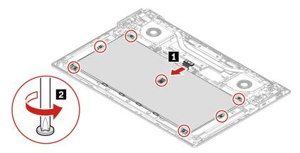
b. Remove the battery as shown below.
