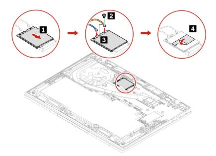
Note: During installation, ensure that you connect the cables with different colors to the corresponding connectors on the module according to the illustrations above: the orange cable to the connector labeled ORANGE, the blue cable to the connector labeled BLUE.
