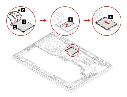
Installation procedure (for wireless WAN card with four antennas)
