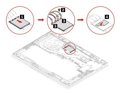
**Note:** During installation, ensure that you connect the cables with different colors to the corresponding connectors on the card according to the illustrations above: the orange cable to the connector labeled ORANGE, the blue cable to the connector labeled BLUE, the white and grey cable to the connector labeled WHITE GREY, and the black and grey cable to the connector labeled BLACK GREY.
