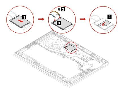
**Note:** During installation, ensure that you connect the cables with different colors to the corresponding connectors on the card according to the illustrations above: the orange cable to the connector labeled ORANGE, the blue cable to the connector labeled BLUE.
