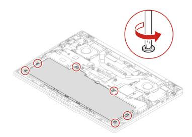
b. Remove the battery as shown below.
