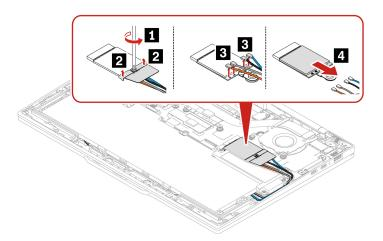
Step 2. Install the captive bracket and wireless WAN module and its bracket in reverse order.
