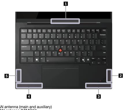
Wireless LAN antenna (main and auxiliary)
