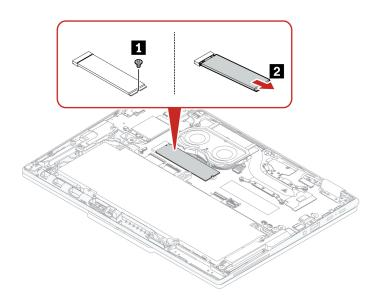
Step 2. Install the M.2 solid-state drive in reverse order.
