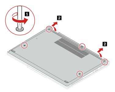
Step 2. Install the base cover assembly as shown below.
