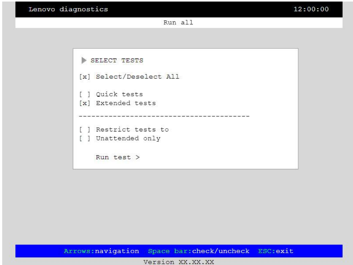
Figure 32 – Run All test
