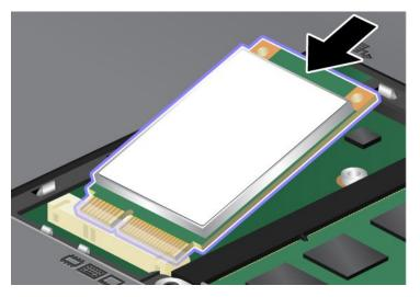
8. Pivot the card downward (1) until you can snap it into place. Secure the card with the screw (2).
