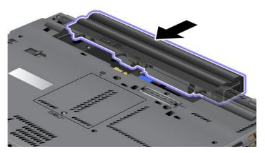
5. Slide the battery latch to the locked position.
