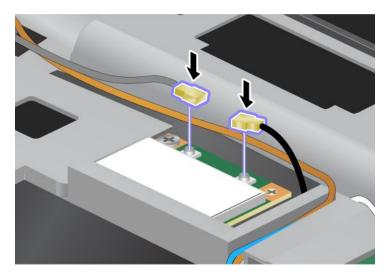
Note: If the new PCI Express Mini Card has three connectors, be sure to attach the gray cable to the connector marked "TR1" on the card, and the black cable to the connector marked "TR2". If you attach either cable to the center connector, the connection speed will be lower.
