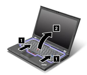
8. Carefully lift the keyboard until you can see how it's connected. Hold the keyboard above the computer, and then detach the connector (1). Now the keyboard has been removed (2).
