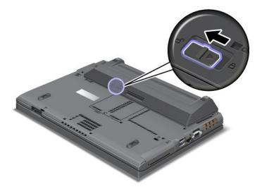
4. Press the latch as shown in the illustration below and detach the battery.
