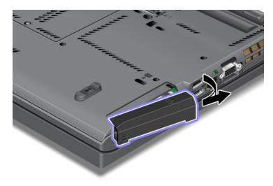
6. Remove the solid state drive by pulling out the tab.
