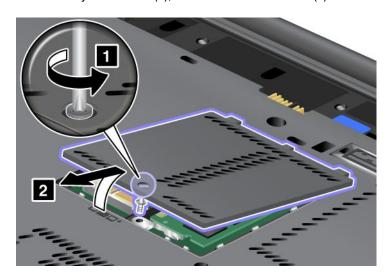
5. Remove the screw that secures the keyboard.
