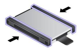
9. Insert the solid state drive into the slot; then press it firmly into place.
