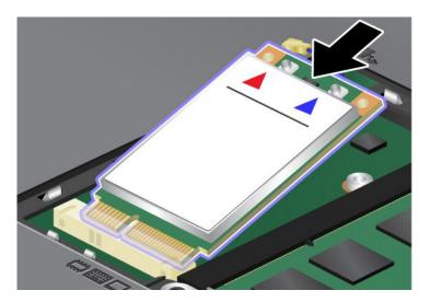
9. Pivot the card until you can snap it into place by pressing the upper side of each connector (1). Secure the card with the screw (2).
