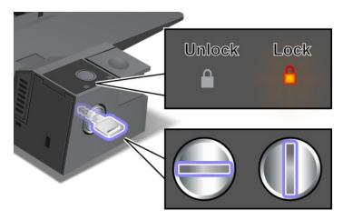
When the key is in the locked position, the eject button of the ThinkPad Mini Dock Series 3, the ThinkPad Mini Dock Plus Series 3, or the ThinkPad Mini Dock Plus Series 3 (170 W) is locked, and you cannot remove your computer. The key lock indicator lights when the eject button is locked.
