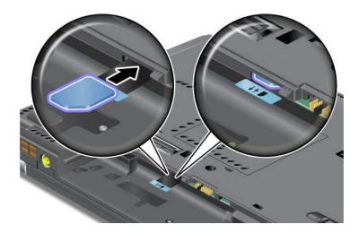
Note: Make sure that you insert the SIM card all the way into the slot.
