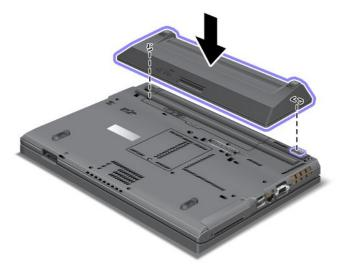
4. Slide the battery latch to the locked position.
