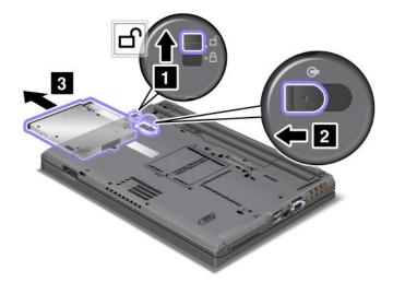
3. Insert the replaceable device into the bay; then press the device firmly into the connector.
