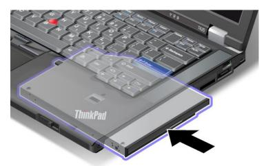
Note: If a hard disk password is set on a hard disk drive, you cannot hot-swap the drive. First remove the hard disk password, and then do the hot swap. Refer to "Hard disk passwords" on page 91.
