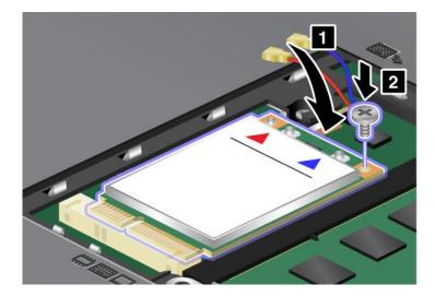
**Note:** Depending on the system configuration of your computer, the card may have only one connector. 10. Connect the cables to the new PCI Express Mini Card (3).
