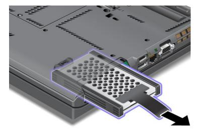
7. Detach the side rubber rails from the hard disk drive.
