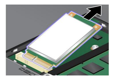
7. Align the contact edge of a new mSATA solid state drive with the corresponding socket.
