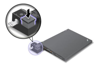
3. Press the eject button (1) until the computer moves up; then, grasping both sides, remove the computer (2).
