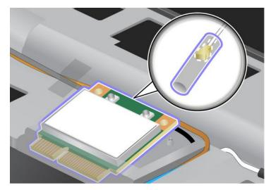
9. Pivot the card until you can snap it into place by pressing the upper side of the connectors (1). Secure the card with the screw (2).
