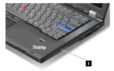
2. Insert the replaceable device into the bay; then press the device firmly into the connector.
