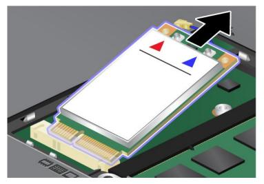
8. Align the contact edge of the new PCI Express Mini Card with the corresponding socket.
