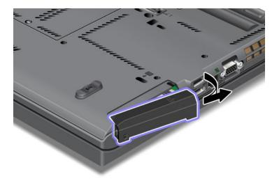
6. Remove the hard disk drive by pulling out the tab.
