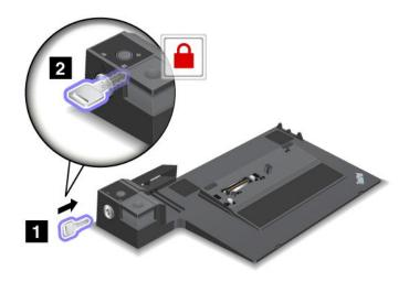
2. Press the button of the ThinkPad Mini Dock Series 3, the ThinkPad Mini Dock Plus Series 3, or the ThinkPad Mini Dock Plus Series 3 (170 W) (1). Pull the sliding adjuster in the direction shown by the arrow (2).
