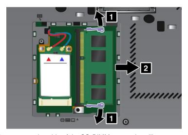
5. Find the notch on the contact edge side of the SO-DIMM you are installing.
