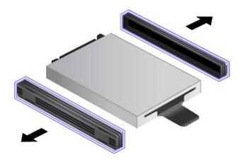
8. Attach the side spacer rails to a new solid state drive.
