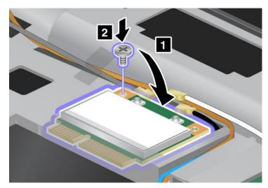
10. Connect the cables to the new PCI Express Mini Card. Be sure to attach the gray cable to the connector marked "TR1" on the card, the white cable to the connector marked "RO" or "TR3" (center), and the black cable to the connector marked "TR2".
