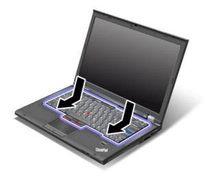
4. Close the computer display, and turn the computer over. Reinstall the screw.
