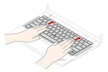
Step 3. Pivot the keyboard slightly upward 11 and then turn over the keyboard 21.
