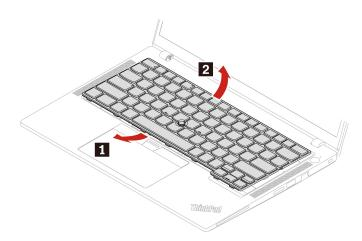
Put the keyboard on the palm rest as shown and detach the connectors. Then, remove the Step 4. keyboard.
