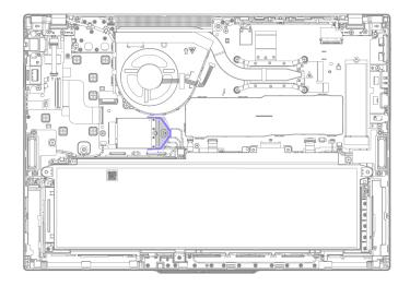
Step 1. Remove the wireless-WAN-module bracket as shown below.
