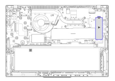
Step 1. Remove the M.2 solid-state drive bracket as shown below.
