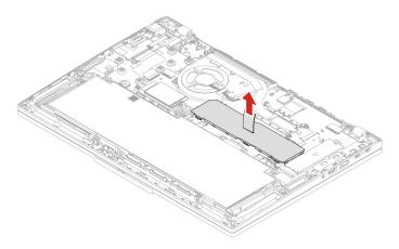
Step 2. Install the memory module shielding cap as shown below. ThinkPad T14 Gen 5 and ThinkPad P14s Gen 5 AMD
