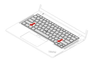
Step 4. Tighten the screws to secure the keyboard.
