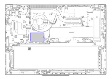
Step 1. Remove the wireless WAN module as shown below.
