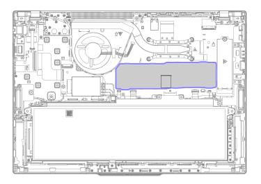
Step 1. Remove the memory module shielding cap as shown below. ThinkPad T14 Gen 5 and ThinkPad P14s Gen 5 AMD
