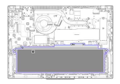
Step 1. Remove the built-in battery as shown below.
