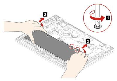
Step 2. Install the built-in battery in reverse order.
