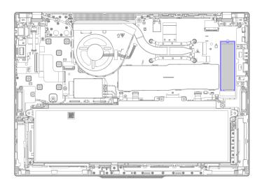
Remove the M.2 solid-state drive as shown below.
