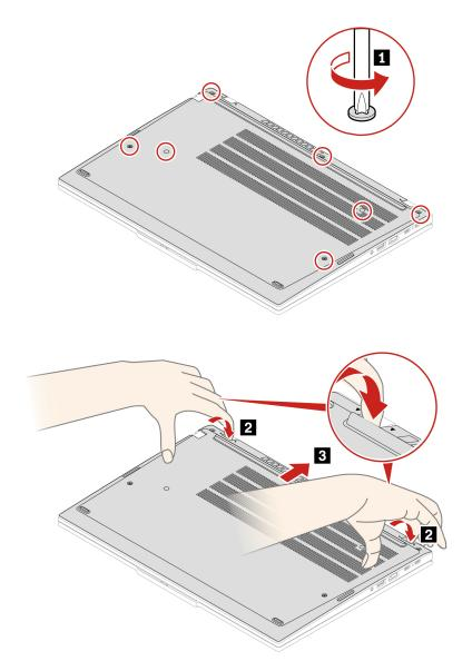
Step 2. Install the base cover assembly as shown below.
