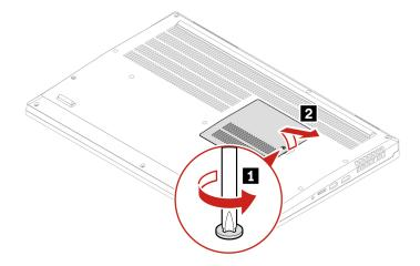
5. Install the new bottom door **1**. Ensure that the latches of the bottom door are secured under the bottom door **2**. Then, tighten the screw to secure the bottom door **3**.
