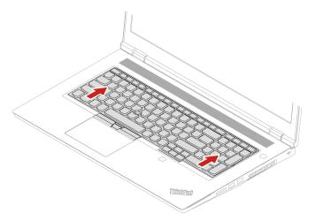
6. Pivot the keyboard slightly upward 1 and then turn over the keyboard 2.
