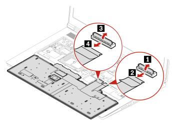
8. Attach the connectors as 1 to 4 shown. Then turn over the keyboard 5.
