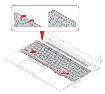
3. Slide the keyboard in the direction as shown. Ensure that the latches are secured under the keyboard frame.
