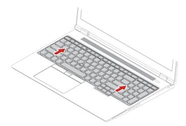
3. Pivot the keyboard slightly upward **1** and then turn the keyboard over **2**.
