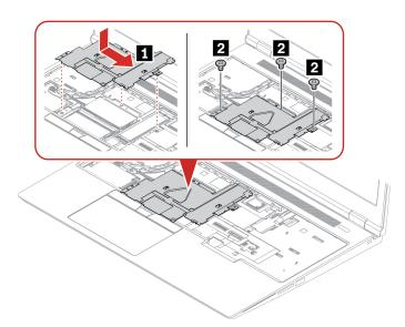
Note: Do not peel off the release paper on the thermal pad when installing the service bracket.
