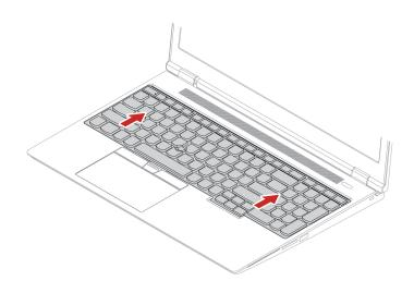
3. Pivot the keyboard slightly upward **I** and then turn the keyboard over **2**.
